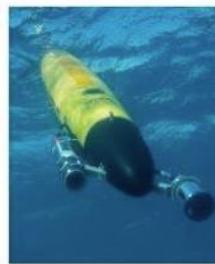
UVP6 on an oceanographic glider
